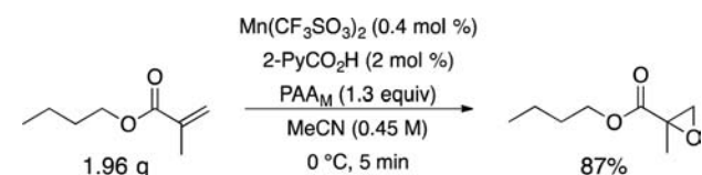
Scheme 1. Gram-scale Synthesis of Butyl 2-Methyl-2-oxiranecarboxylate
